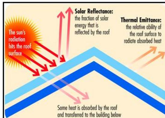
Typical dark roofs can absorb 90% or more of incoming solar energy, while cool roofs may absorb less than 50%. *Image Source: CRRC*
